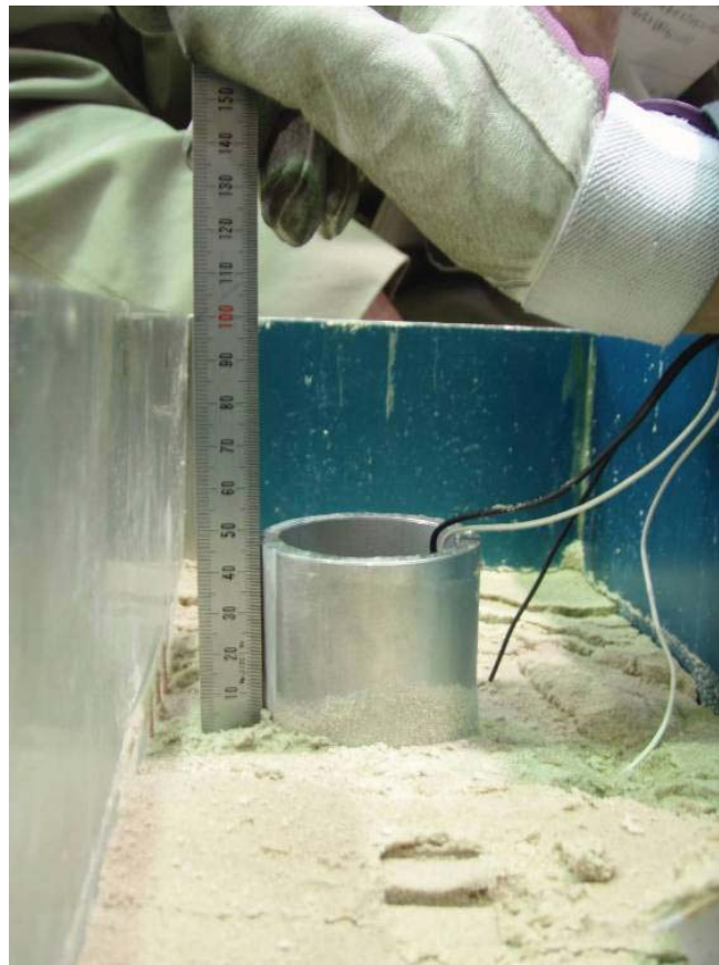
Fig. 2.8 Uplifted manhole after shaking (CS2).
