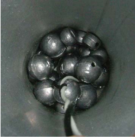
Fig. 2.22 Lead beads using the centrifuge model tests to increase an apparent unit weight of the manhole.
