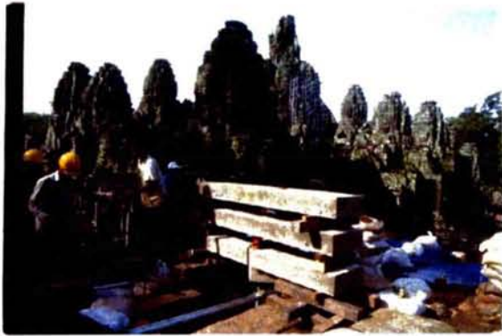
Photo 8-13 Plate Loading Test
