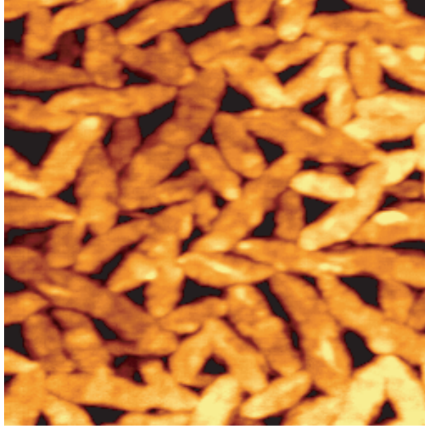
Figure 3.5: The AM-DFM image of the P(VDF/TrFE) thin film annealed at 140°C for 2 h ( 1\ \mu\text{m} \times 1\ \mu\text{m} ).
