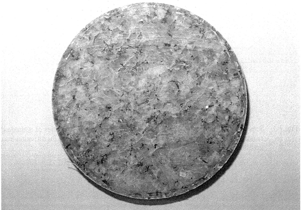
Fig. 7-2a Autoradiographic and optical images for the "hot" side of the granite disk, F3 used in the 1 st series of diffusion experiment for actinide carbonate complexes.
