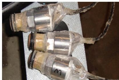
Figure 2.7 Pressure transducers
