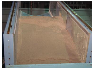
Figure 2.20 Observed slope sliding (23° flume slope - Experiment D)
