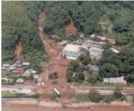
Figure 1.8 Slope failure due to torrential rainfall of the Bai-u front (Hanakura Area, Kagoshima City, Kagoshima Prefecture August 6, 1993) (*Photo Courtesy: MLIT, Japan*)
