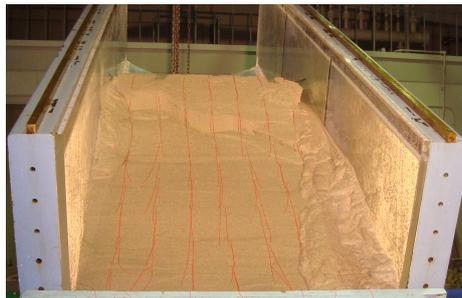
Figure 2.21 Observed slope sliding ( $23^\circ$  flume slope - Experiment E)
