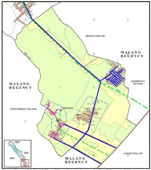
Figure 3.9 Piped Clean Water Supply System in Candi Renggo Village Note: Blue solid line is main pipeline of PDAM, magenta dash line is main pipeline of HIPPAM, and green dash line is main pipeline of Indonesian Military and Education Institution
