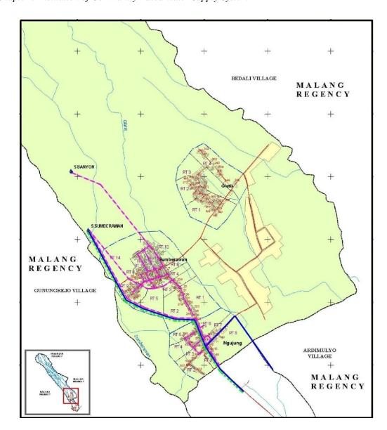
Figure 3.8 Piped Clean Water Supply System in Toyomarto Village Note: Blue solid line is main pipeline of PDAM, magenta dash line is main pipeline of HIPPAM, and green dash line is main pipeline of Indonesian Military and Education Institution
