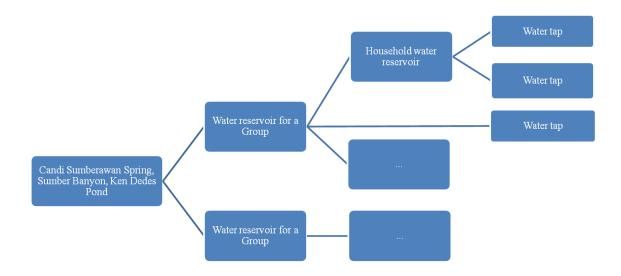
Figure 3.6 Piped Clean Water Supply System from HIPPAM
