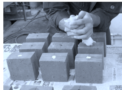
Figure 4.2: Application of impregnant (water penetration barrier agent).
