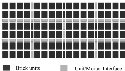
Figure 3.22: Masonry unit and unit/mortar interface discretization.
