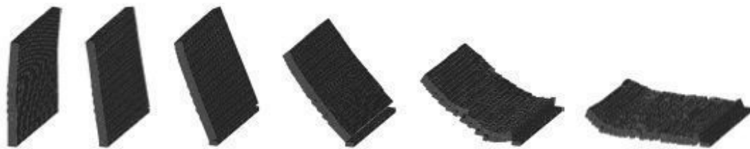
Figure 2.27: Collapse behavior sequence of wall with discrete element model [40].
