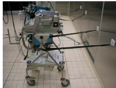
(b) Equipment attached by longer belts to the wall
