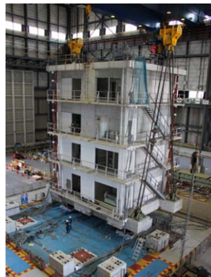
Figure 3-5 Lifting the specimen to set on the shaking table
