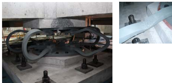
Figure 4-3 U-shaped steel damper after all shakings (Test II)
