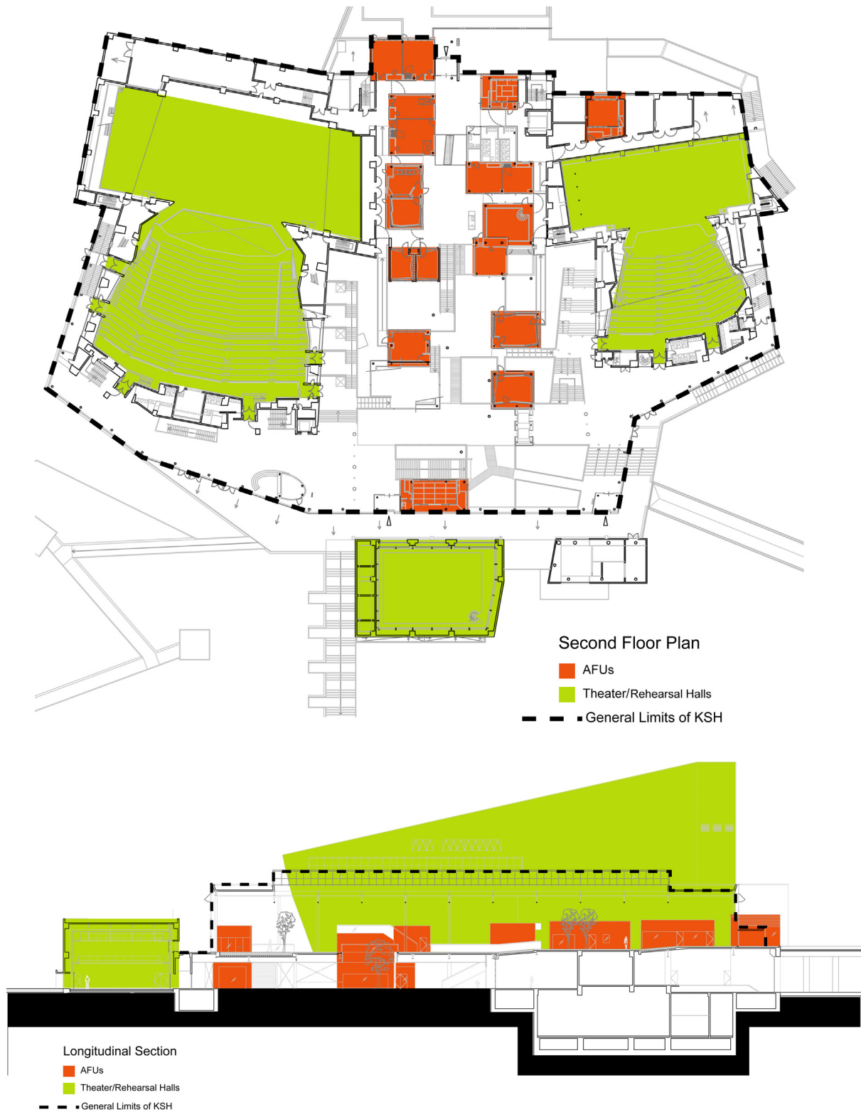
Figure 5.18 Second Floor Plan (top) and Longitudinal Section (bottom) of Kitakami Sakura Hall
