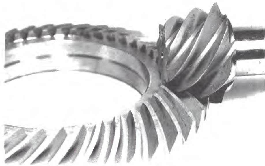
(a) Photograph of tooth bearing
