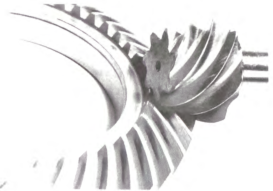
(a) Photograph of tooth bearing
