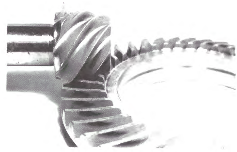
(a) Photograph of tooth bearing
