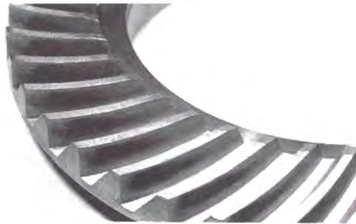
(a) Photograph of tooth bearing
