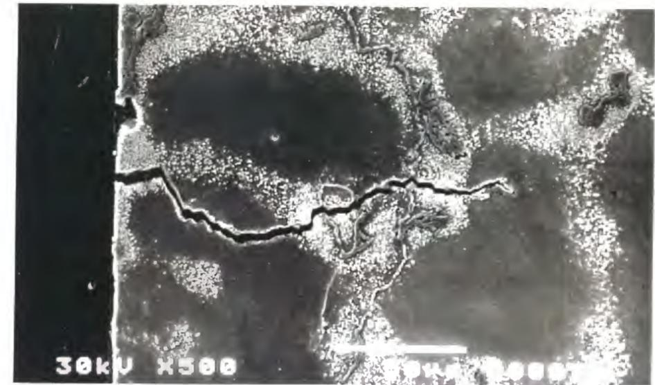
Fig.2.20 Observation of HTLCF specimen section by SEM for FSX414 tested at 1023K.
