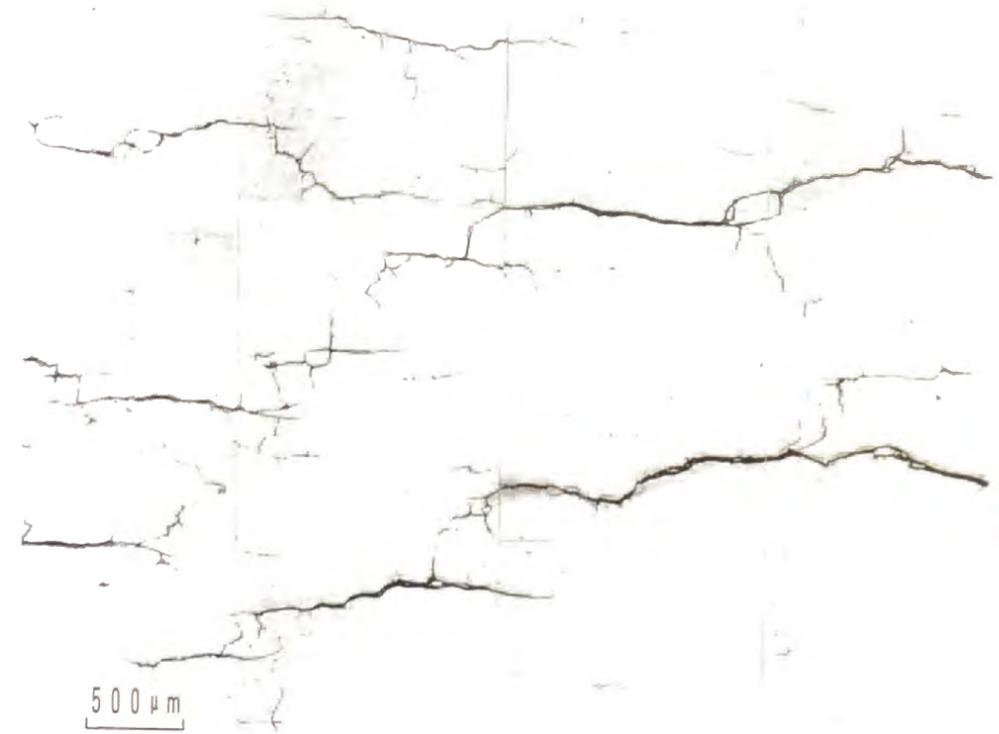
Fig.3.10 Specimen surface replica observation for HTLCF damaged Nimonic263 after 450 cycles ( $N/N_{25}=0.92$ ,  $\Delta\varepsilon_f=1\%$ ,  $T=1123\text{K}$ , before etching).
