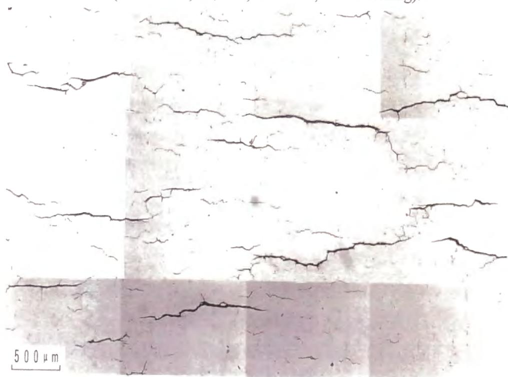
Fig.3.9 Specimen surface replica observation for HTLCF damaged Nimonic263 after 300cycles ( $N/N_{25}=0.61$ ,  $\Delta\varepsilon_f=1\%$ ,  $T=1123\text{K}$ , before etching).
