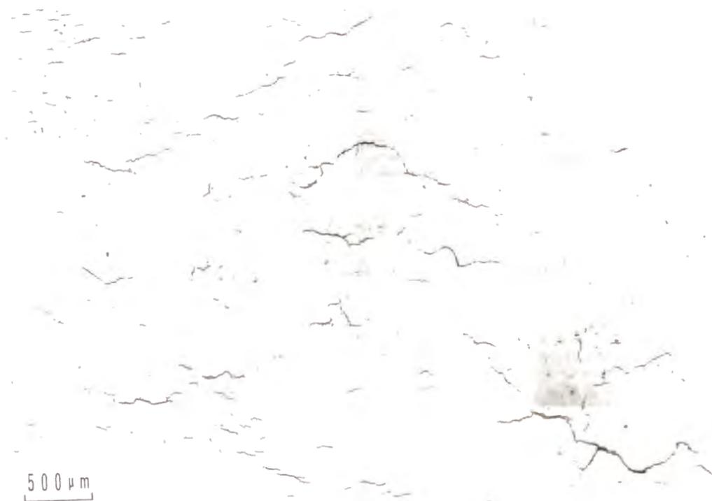
Fig.3.2 Specimen surface replica observation for HTLCF damaged FSX414 after 200cycles
