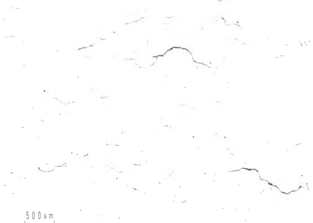
Fig.3.3 Specimen surface replica observation for HTLCF damaged FSX414 after 300cycles
