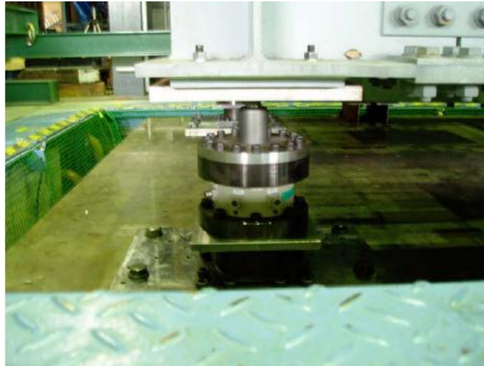
Figure 5.11 Pure friction bearing
