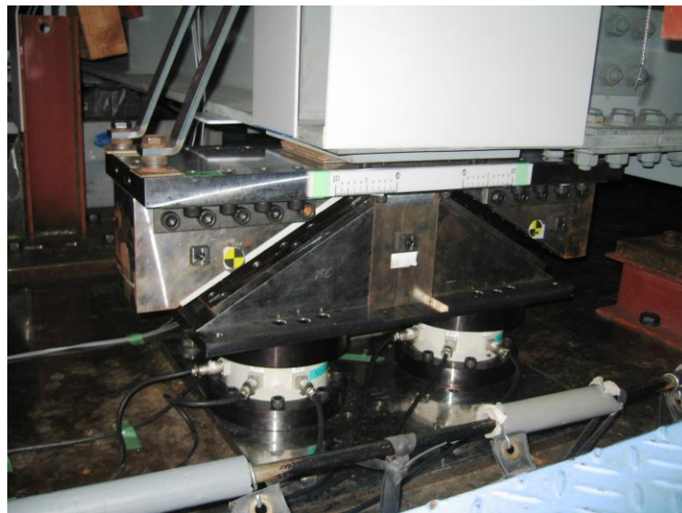
Figure 5.10 Uplifting sliding bearing
