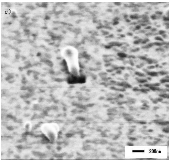
Figure 2.9 SIM images of pillar array: (a) before cutting with FIB (b) after cutting with FIB and (c) tilted at an angle of 60^\circ .
