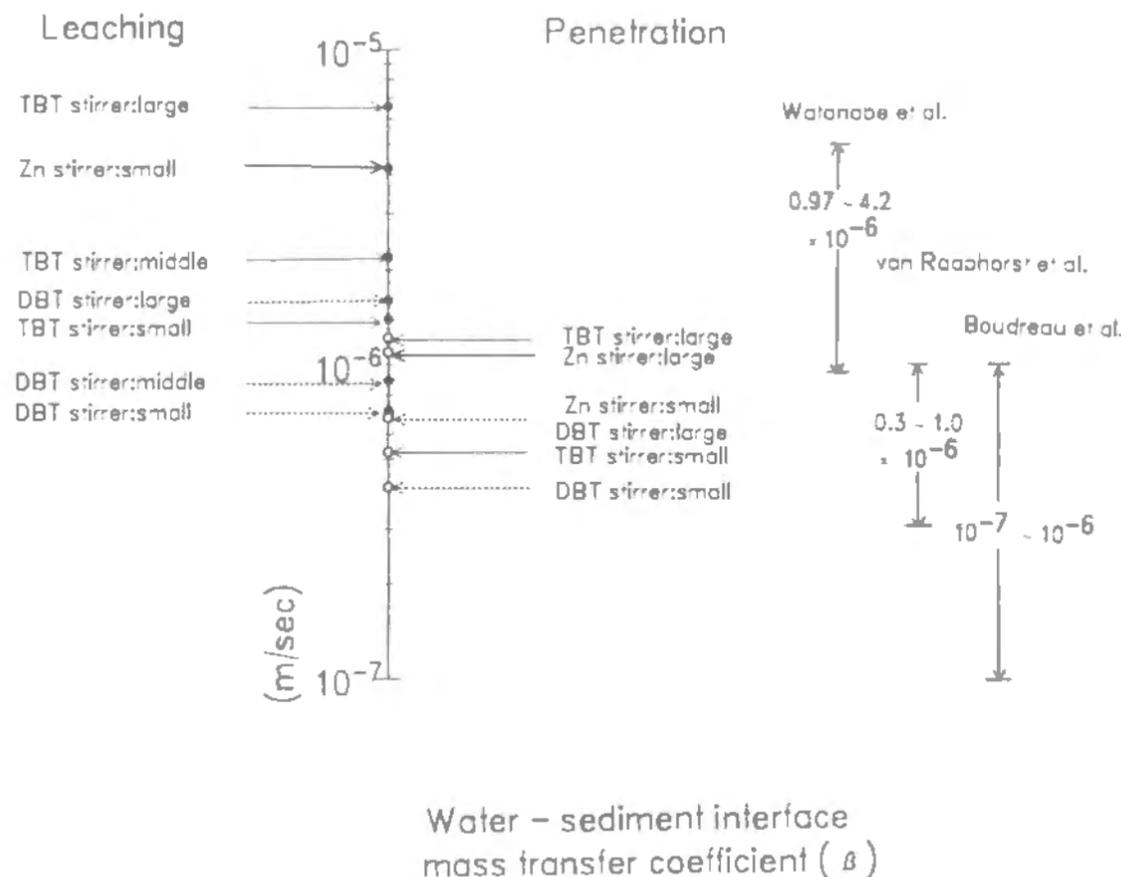
Water - sediment interface mass transfer coefficient ( $\beta$ )
