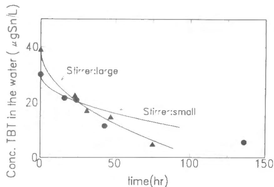
$$\begin{aligned} \text{Stirrer:small } C &= 29.9 - 1.97t^{0.5} \\ \text{Stirrer:large } C &= 39.0 - 3.80t^{0.5} \end{aligned}$$
