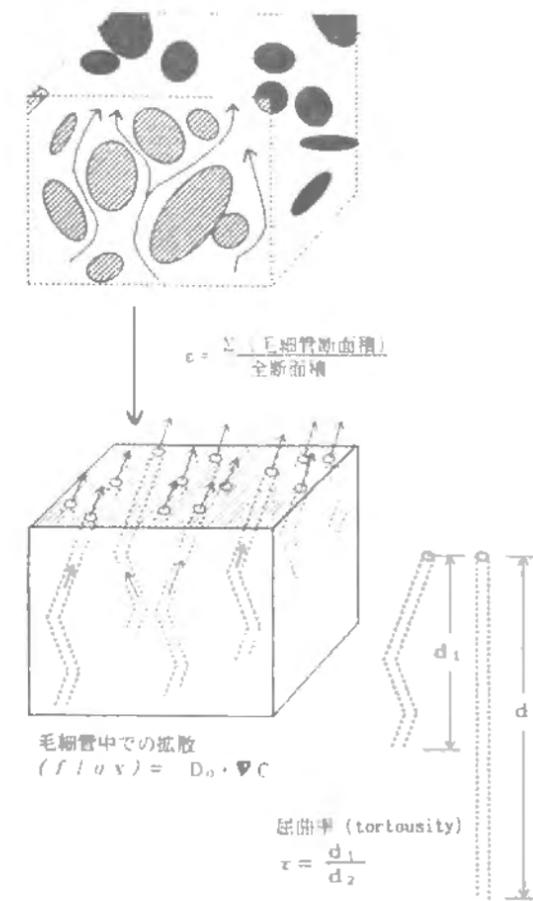
$$(flux) = D_0 \frac{\partial C}{\partial z} \times \varepsilon \times \frac{1}{\tau} = \frac{\varepsilon}{\tau} D_0 \frac{\partial C}{\partial z} = D_i \frac{\partial C}{\partial z}$$
