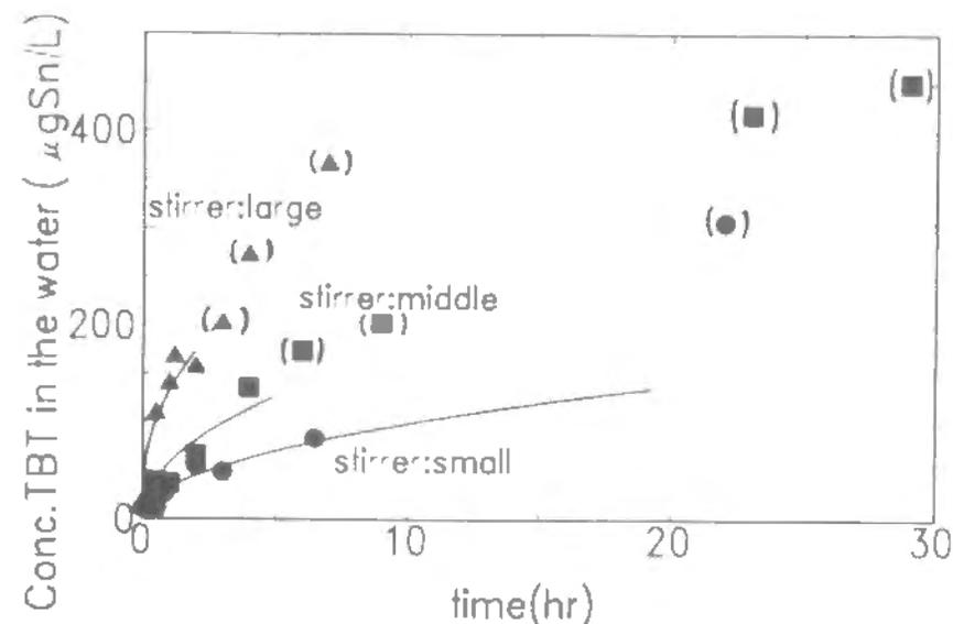
$$\begin{aligned} \text{Stirrer:small } C &= 1.4 + 31t^{0.5} \\ \text{Stirrer:middle } C &= 1.4 + 56t^{0.5} \\ \text{Stirrer:large } C &= 9.3 + 127t^{0.5} \end{aligned}$$
