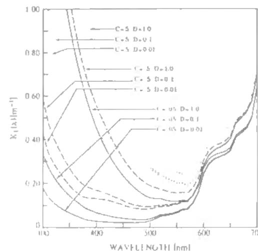
Spectral diffuse attenuation coefficient vs. wavelength for a range of chlorophylls (mg pigment  $m^{-3}$ ) and dissolved organic material (mg DOM liter<sup>-1</sup>) calculated using model as summarized in Tables 2 and 3.
