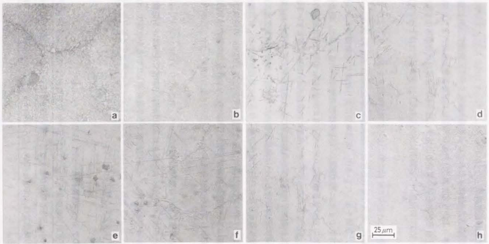
Fig.3.8 IN738LC 時効材の光学顕微鏡観察結果 850°C時効 : (a)0h 材, (b)1000h 材, (c)10000h 材, (d)24000h 材 24000h 時効 : (e)750°C材, (f)800°C材, (g)850°C材, (h)900°C材
