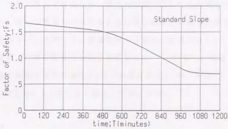
図5.5 標準斜面の斜面安全率 (Fs) の推移 Fig.5.5 Fluctuation of safety factor (Fs) of the standard slope.
