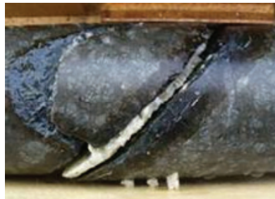
Fig. 3.7: A serpentinite core sample with carbonate at Hidaka, Hokkaido (after RITE, 2008).
