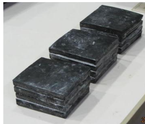
Figure 5.5 Fully cured bonded STRP-4
