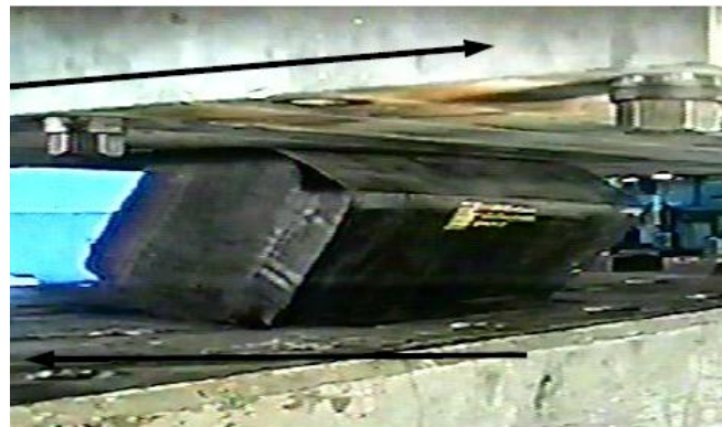
Figure 2.1 Steel laminated elastomeric bearing without fastening system
