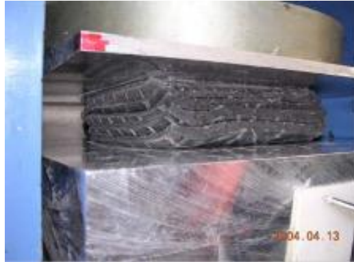
Figure 2.9 Test setup with scrap tire pads
