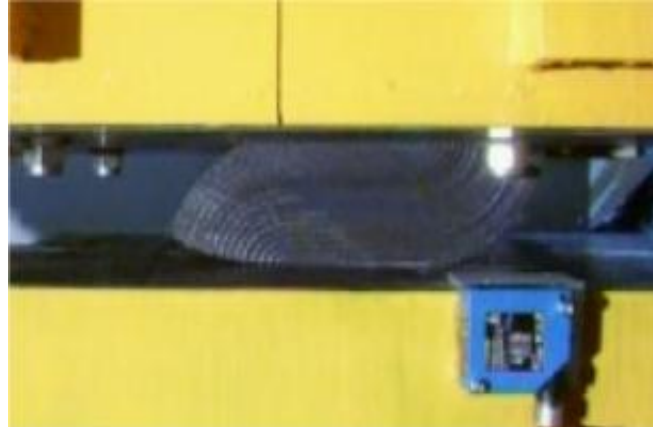
Figure 2.4 Deformed state of fiber reinforced elastomeric isolator at 200% shear strain
