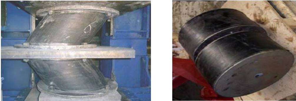
Figure 2.5 New rubber bearings used in Pestalozzi elementary school, Skopje
