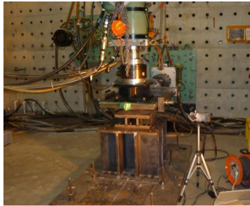
Figure 4.2 Photograph of test setup and instrumentation arrangement
