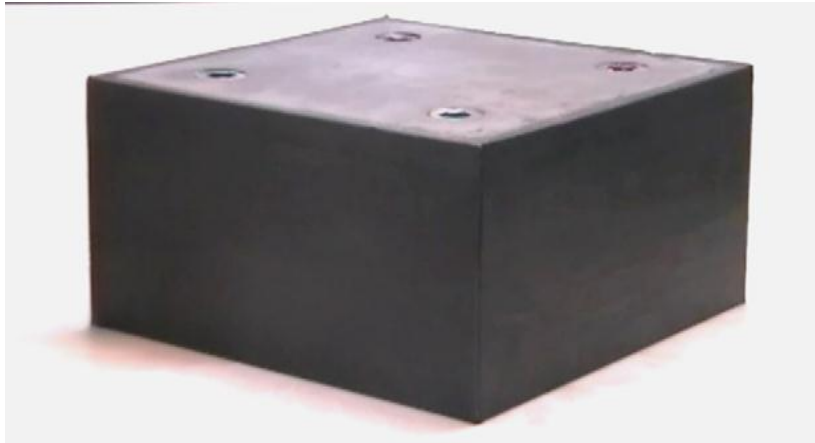
Figure 2.8 1/4 scale fiber reinforced elastomeric isolator
