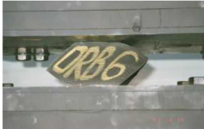
Figure 2.2 Deformed state of fiber reinforced elastomeric isolator at 100% shear strain
