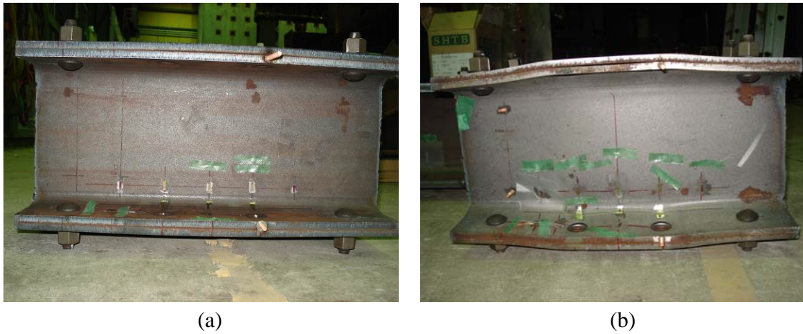
Figure 5.6 Residual deformation: (a) HT-120; (b) CT-120.
