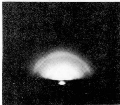
Fig. 5.7 RHEED patterns of the carbon film deposited by (a) the C^- and (b) the C_2^- ion beams at room temperature. (c) RHEED pattern of the carbon film deposited by the C^- ion beam at 800 °C.
