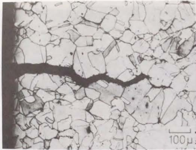
Fig. 7-10 An optical micrograph of the secondary crack appeared near the specimen surface in CP test in air (SUS304, T=800^{\circ}\text{C} , \Delta\varepsilon_t=0.6\% , \Delta\varepsilon_{pp}=0.13\% , \Delta\varepsilon_{cp}=0.31\% )
