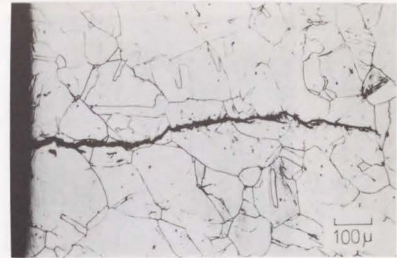
Fig. 7-2 An optical micrograph of the secondary cracks appeared near the specimen surface in PP test (SUS304, T=700°C in air, \Delta \epsilon_t=1\% , \Delta \epsilon_{pp}=0.71\% )
