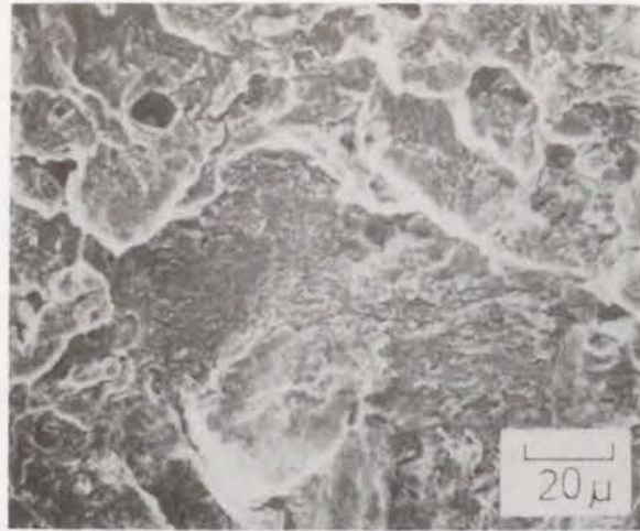
Fig. 7-4 A scanning electron micrograph of the fracture surface obtained in PP test in vacuum (SUS304, T=800^{\circ}\text{C} , \Delta\varepsilon_t=1\% , \Delta\varepsilon_{pp}=0.77\% )
