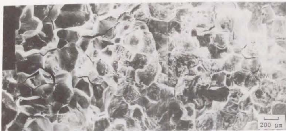
Fig. 9-6 SEM observation of the bowl crack of 1A2-CV
