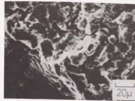
Fig. 7-16 A scanning electron micrograph taken from fatigue-to-creep transition region in the fracture of DC tested specimen (SUS 321, T=650°C, \sigma=18\text{kgf/mm}^2 , t_c=190\text{hr} , \Delta \epsilon_c=1\% , N_f=180 , fractured during 3rd creep period)
