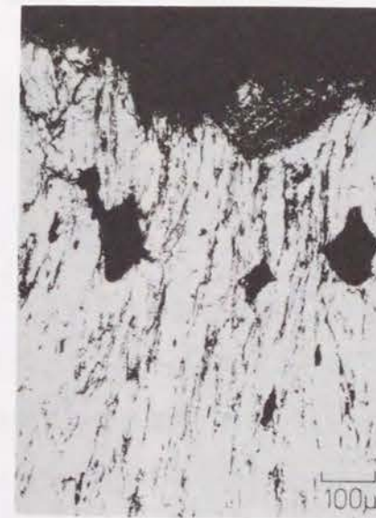
Fig. 7-6 An optical micrograph of longitudinal cross section of the specimen after PC test in vacuum (SUS304, T=700^{\circ}\text{C} , \Delta\varepsilon_t=1\% , \Delta\varepsilon_{pp}=0.53\% , \Delta\varepsilon_{pc}=0.22\% )
