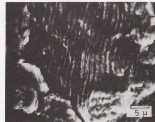
Fig. 7-3 A scanning electron micrograph of the fracture surface obtained in PP test in air (SUS321, T=650°C, \Delta \epsilon_t=0.6\% , \Delta \epsilon_{pp}=0.27\% )
