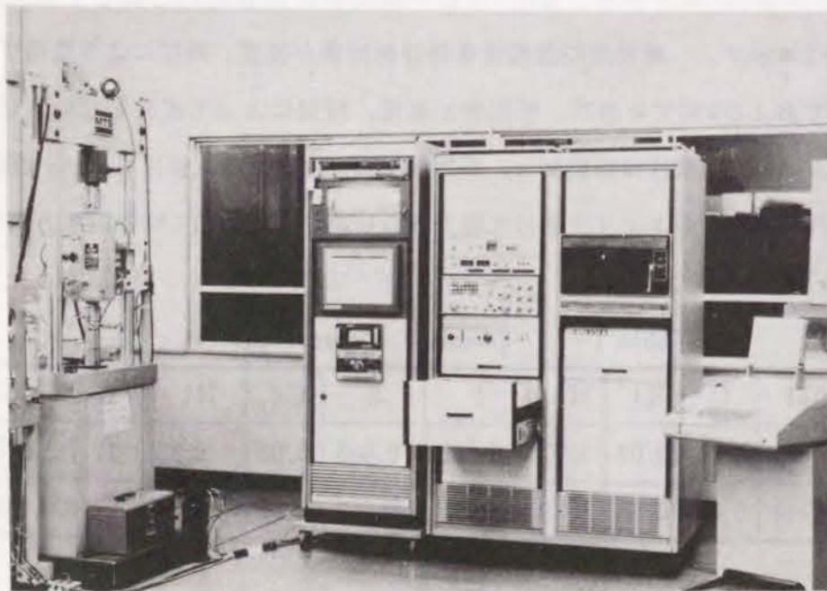
Fig. 1-1. High temperature low-cycle fatigue testing apparatus
