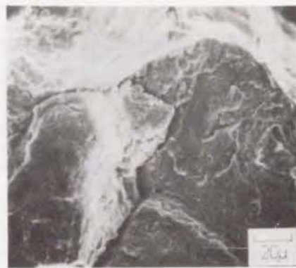
(b) At the center of the fracture surface ( T=650^{\circ}\text{C} , in air)
