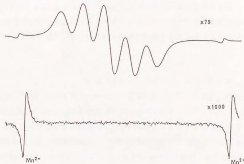
Figure 13. ESR spectrum of DPPH (0.52mM) before (A) and after (B) the addition of CV-6504 hydroquinone (1.0mM).
