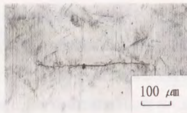
(a) A pre-crack introduced by fatigue at room temperature.
