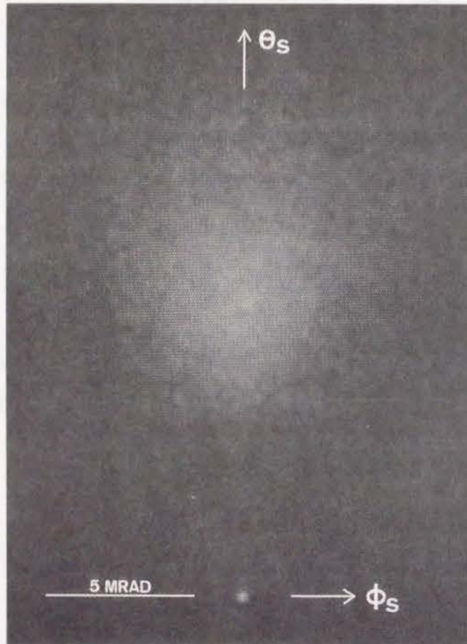
Figure 3.5: Angular distribution of scattered He ions from the (100) surface of SnTe at the incidence of 0.7 MeV He + with glancing angle 4.6 mrad. Specular reflection (incidence along random direction). Bright spots at bottom of patterns are the residual incident beam. \theta_s - and \phi_s -axes are shown.
