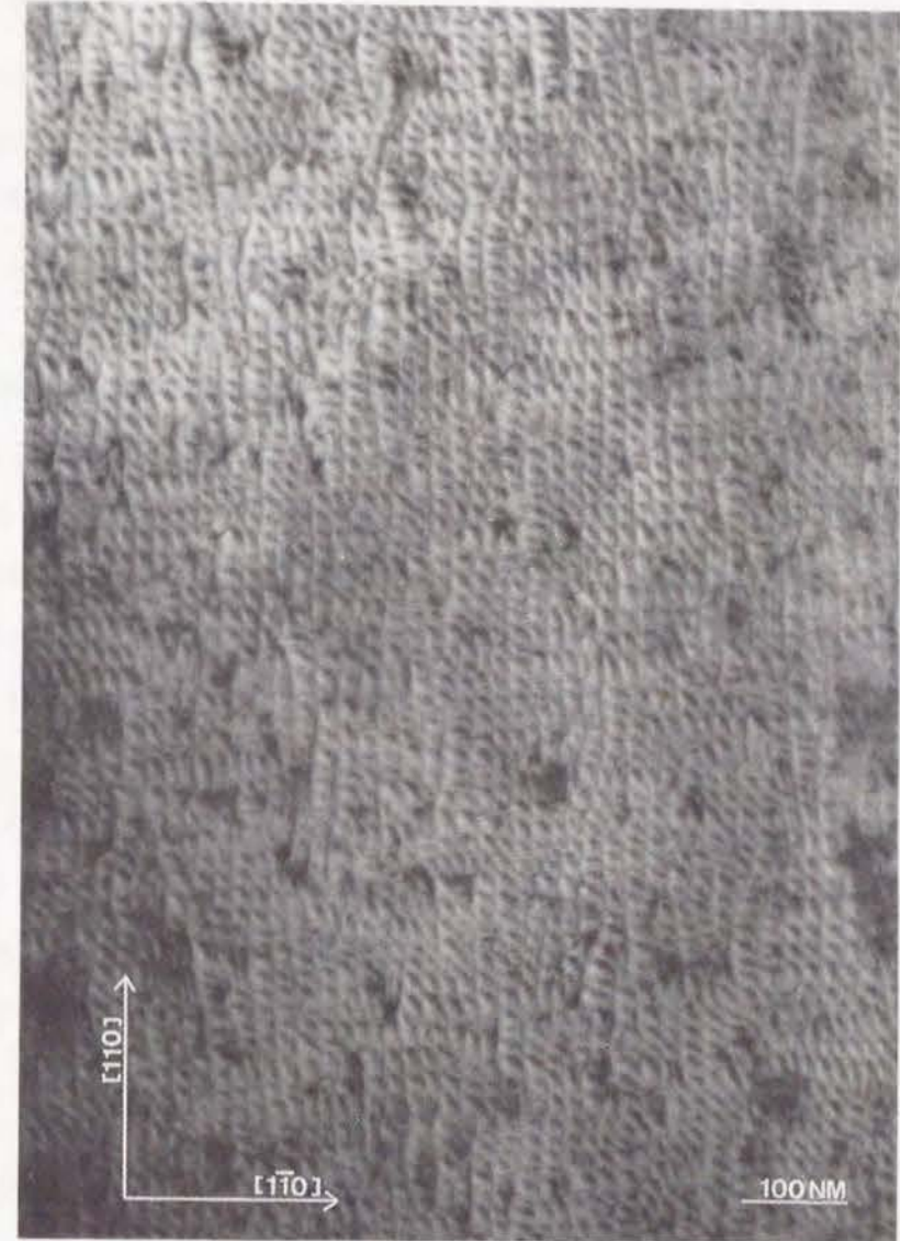
Figure 9.2: An electron micrograph of PbSe/SnTe bicrystal, where PbSe is 3 nm thick. Dislocations are parallel to the \langle 110 \rangle axes on the (001) interface.
