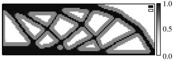
Figure 3.7: Configuration using the proposed MPPM before removing grayscales.
