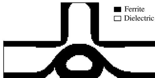
Figure 7.14: Optimized configuration of T-junction design problem.
