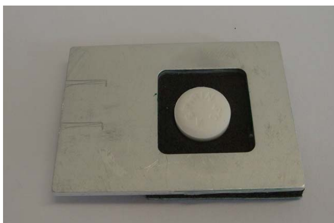
Photo. 2.1 A tablet analgesic antipyretic drug on an Al sample holder.
