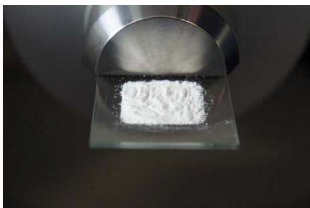
Photo. 2.2 Powdered analgesic antipyretic drug placed loosely on a glass sample holder.
