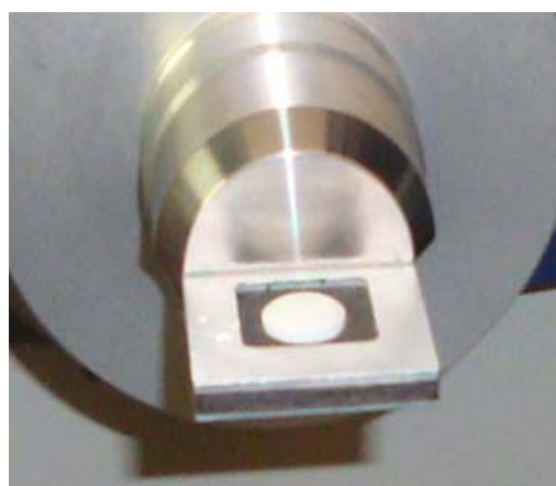
Photo. 2.1 A tablet analgesic antipyretic drug on an Al sample holder.
