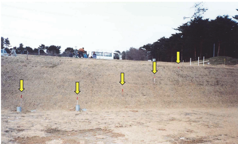
Fig.1.4-2 Photograph of the experimental site. Steel pipes were buried at the stakes which head colored red.
