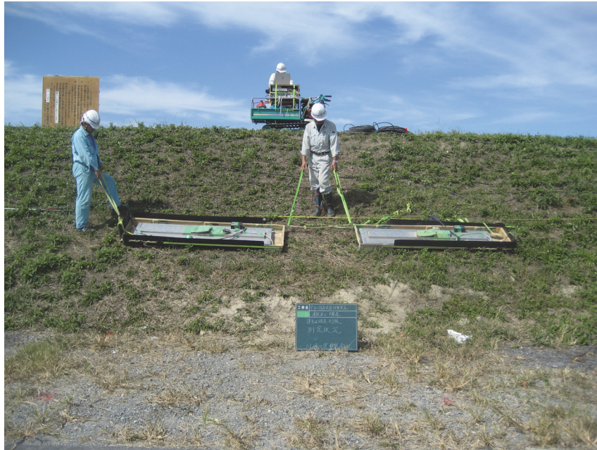
Fig.2.3-5 Photograph of the pseudo-three dimensional measurement at Uji river embankment.
