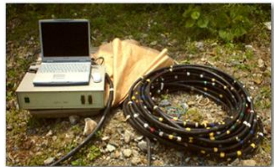
Fig. 6. The instrument of the Multipoint Temperature Logging method
