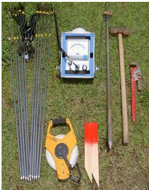
Fig. 1. The instrument of One-meter Depth Temperature method Fig. 2. Process of operation
