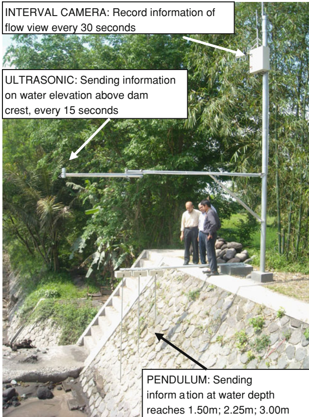
Fig. 12 Cross-sectional monitoring system at Rejodani
