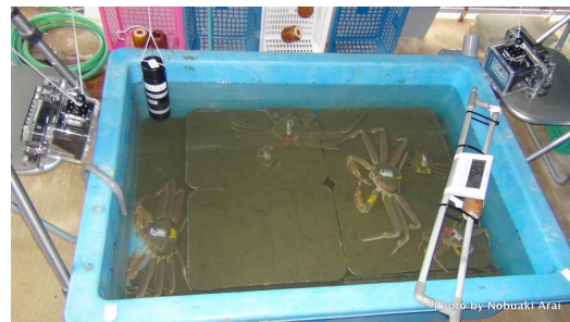
Fig. 1 Five snow crabs were placed in a 300-L tank with chilled seawater, which was fitted with an acoustic receiver (VR2W) and covered with mud in the bottom. The infrared projectors of both sides were used at night.
