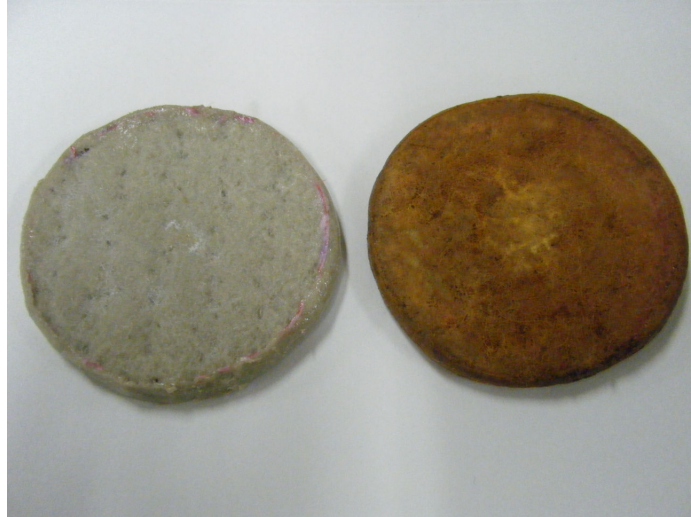
Figure 4-24 GCL after hydraulic conductivity test: water permeation (left), ARD permeation (right)
