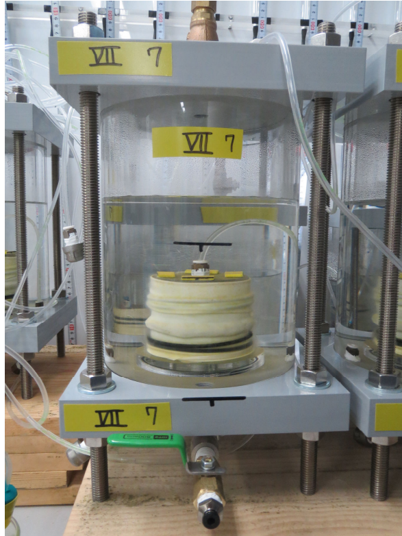
Figure 4-8 System used to measure the hydraulic conductivity of GCL
