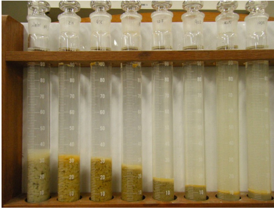
Figure 4-5 Swelling test of different ARD dilutions
