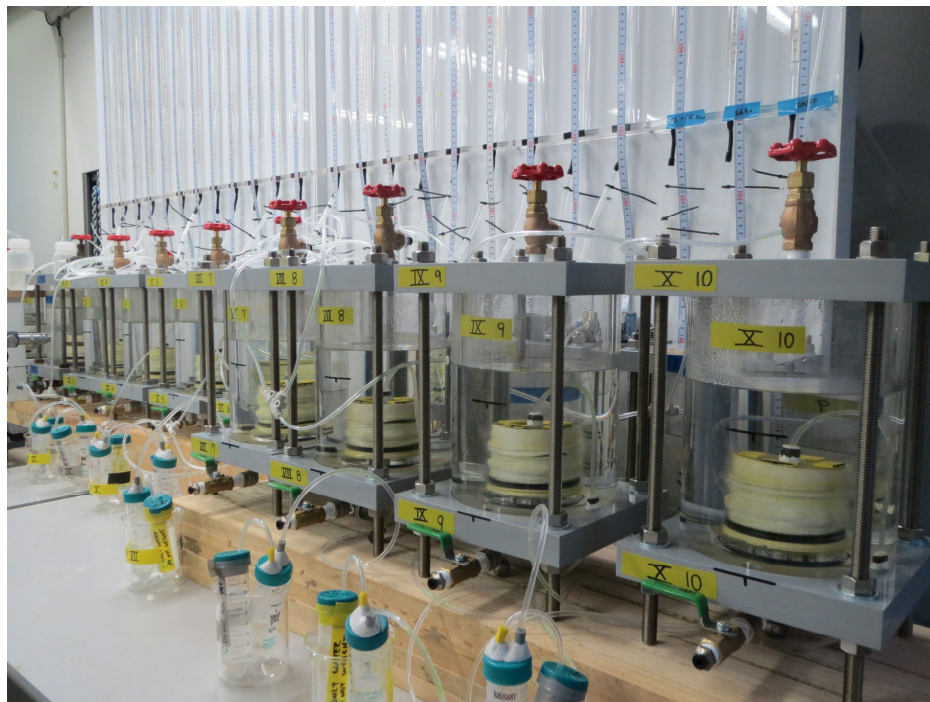
Figure 4-7 Equipment used to evaluate the hydraulic conductivity
