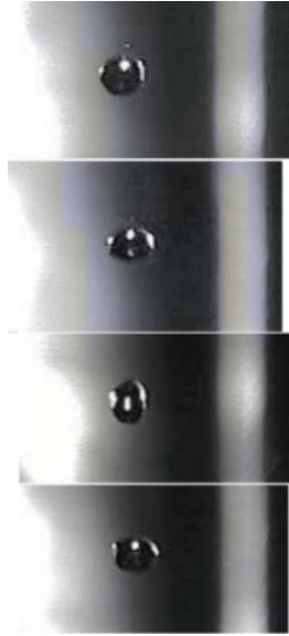
Fig. 6, Oscillating deformation of one droplet, recorded with high speed video camera. Frequency was approximately 200 Hz.
