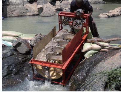
Fig. 9. Screw turbine pico-hydro system setup
