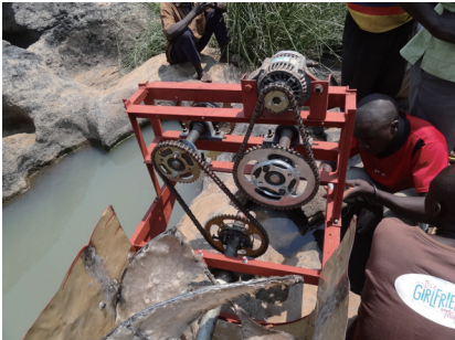
Fig. 6. Transmission of the screw turbine
