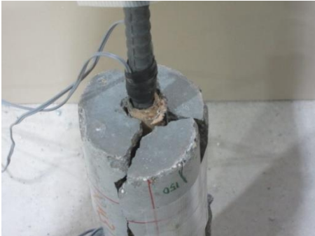
Photo 5.4 Specimen having splitting failure
