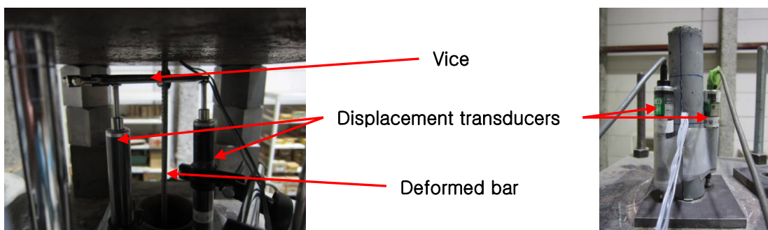
Photo 5.3 Set up of pull-out test
