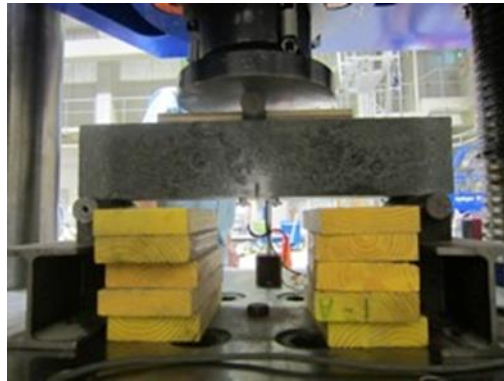
Photo 3.3 Three point flexural test
