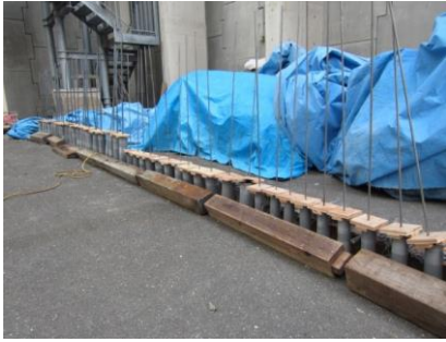
Photo 5.1 NM and PCM specimens for pull-out test
