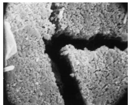
Portland cement concrete
