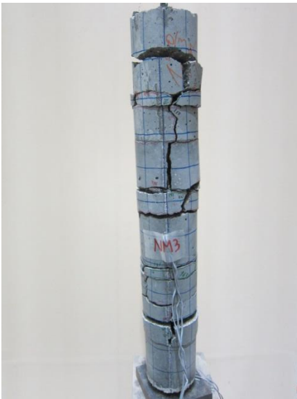
Photo 5.10 Specimen having many cracks
