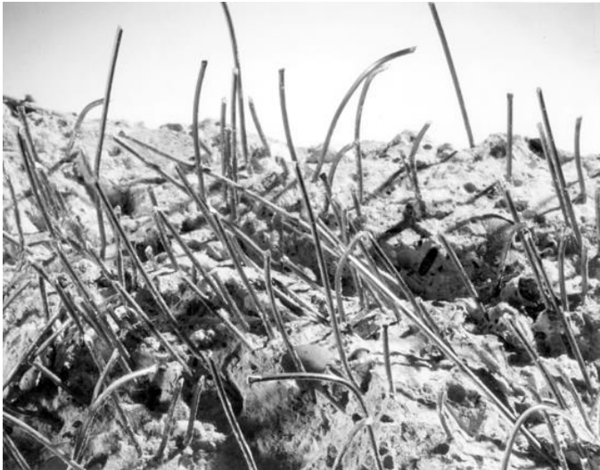
Figure 2.1 Fracture surface of steel fiber reinforced concrete (ACI committee 544 1996)
