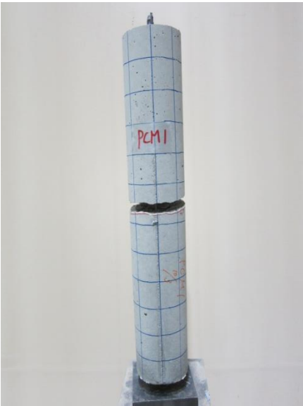
Photo 5.9 Specimen having a few cracks
