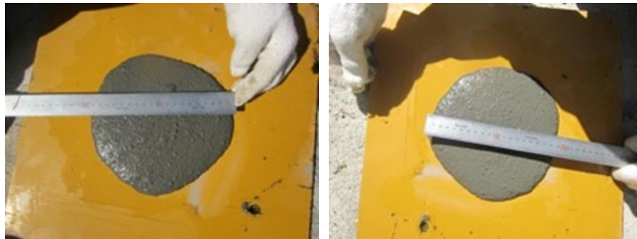
Photo 3.4 Flow of NM (190 X 200mm)
