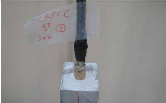
Photo 5.5 Specimen that steel bar was pulled out
