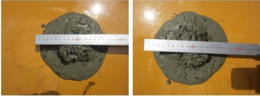
Photo 3.9 Flow of SCP (190 X 190mm)
