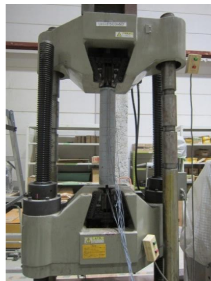
Photo 5.8 Set up of uniaxial tension test
