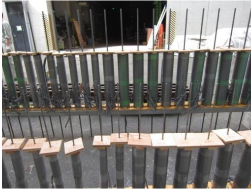
Photo 5.6 NM and PCM specimens for uniaxial tension test
