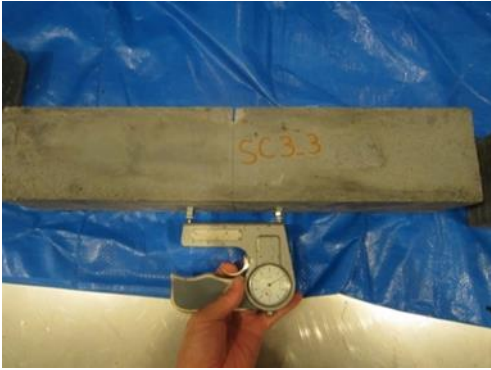
Photo 6.1 Strain measurement with a contact gauge
