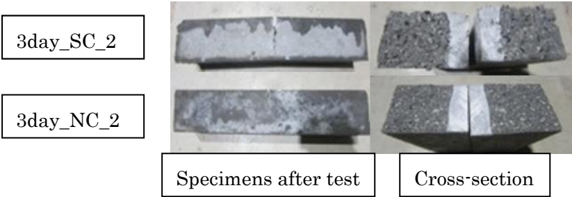
Photo 3.7 Specimens after flexural strength test
