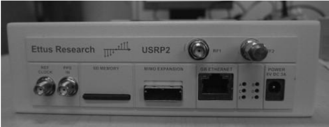
FIGURE 2.6: A view of the USRP2 interface.
