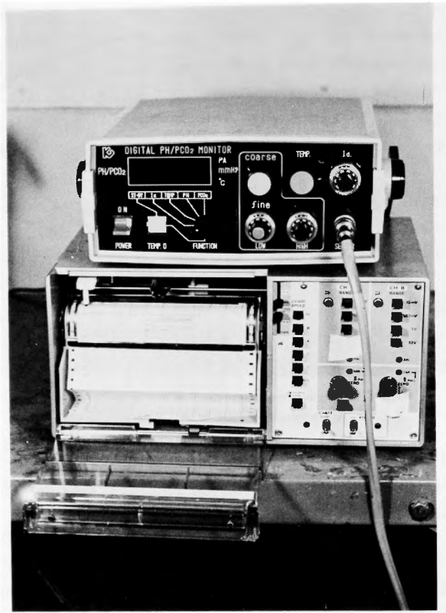
Fig. 3. KR. 500 pH/pCO 2 monitor (above) and KR-102 pen recorder (below).
