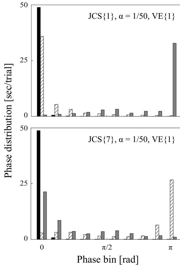
**Figure 2:** Two examples of phase distribution. Phase difference between two adjacent joints is separated into ten bins. The sum of each colored bar is 50 s (the whole trial length). Black, hatched, and gray bars represent MP-ankle, ankle-knee, and knee-hip phase distributions, respectively. Each parameter conditions are shown in the top-right corner of each figure.
