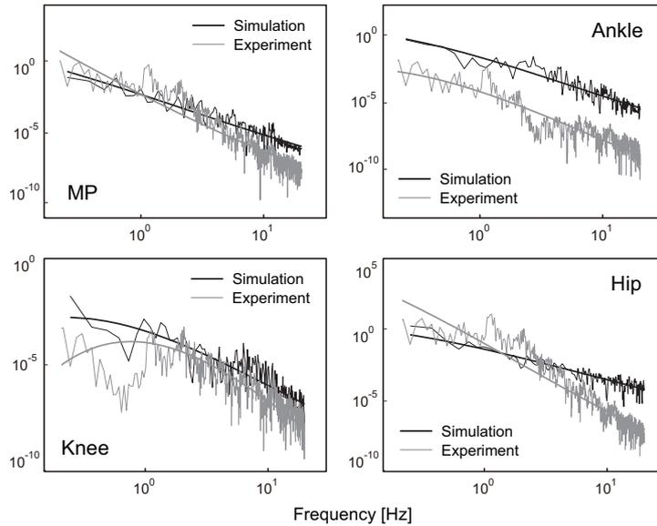
**Figure 7:** Comparison in the power spectrum of angular displacements between simulation and experiment. Black and gray lines are the logarithm plots of the power spectrum of each angular displacement for simulation and experiment, respectively. The power spectrum was shown up to 20 Hz, which is physiologically relevant range of frequency component of joint oscillations.
