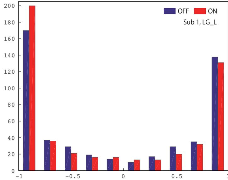
**Figure 5:** Sample DC histogram. Red and blue bar represent DC of on-points and off-points, respectively, during a 120-sec trial (LG of subject no. 1). DC of 1 and -1 means that the actual state point moves forward and against the model dynamics of a triple inverted pendulum, respectively.
