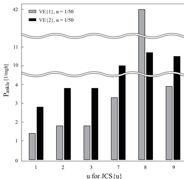
**Figure 3:** Stability region of the ankle gain  $P$  for six JCS pairs. Each  $JCS\{u\}$  corresponds to the ones shown in Table 2. Gray and black bars represent two different viscoelasticity parameters shown in the top-left corner. The minimum  $P$  value was 0.1 for all conditions.
