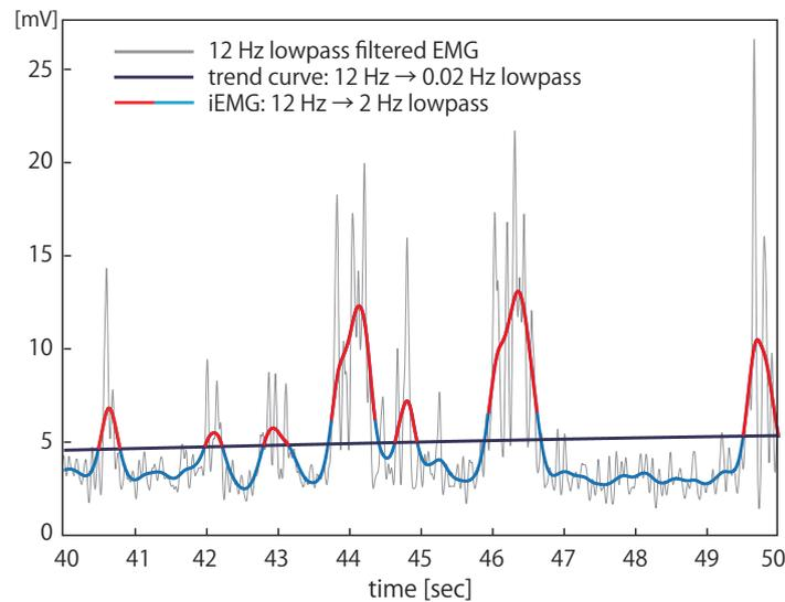
**Figure 1:** Muscle activation/inactivation (on/off) discrimination. Sample EMG signal is shown. Gray plot represents 12 Hz low-pass filtered EMG signal after full wave rectification. Dark blue plot is a trend curve, which is 0.02 Hz low-pass filtered EMG signal. 2 Hz low-pass filtered iEMG signal is consisted of red and light blue curves, which represent muscle activation and inactivation, respectively.
