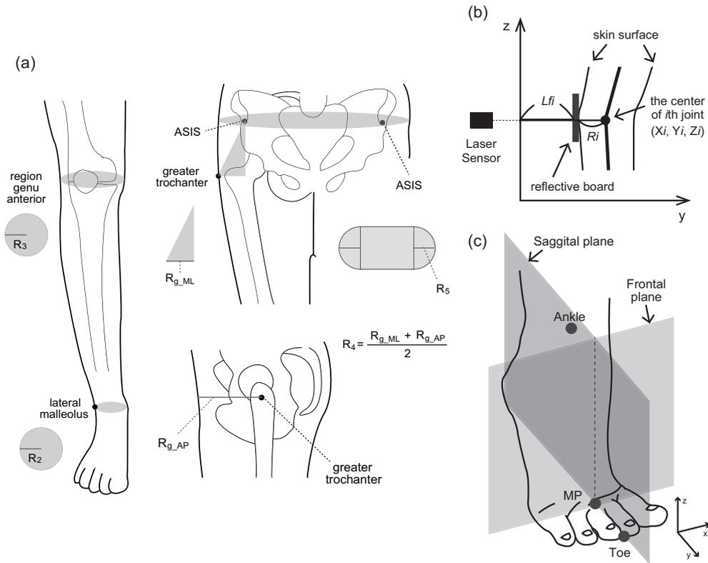
**Figure 3:** The coordinates of the center of joints and segment-specific sagittal and frontal planes. (a) Radii of the ankle, knee, and hip (greater trochanter) and the depth of the anterior superior iliac spine (ASIS). The ankle and knee were approximated to circles, whose radii were  $R_2$  and  $R_3$ , respectively. The radius of hip ( $R_4$ ) was defined to be the mean of its anterior depth and the horizontal distance between greater trochanter and ASIS. The horizontal plane
