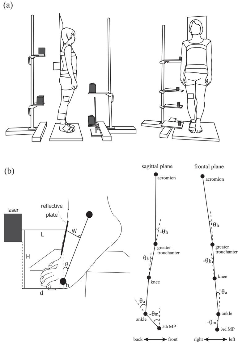
**Figure 1:** Experimental set up and parameters for the analysis. (a) Experimental setup. Each joint's displacement was measured by eight laser sensors. (b) Parameters for the data analysis. The left and right figures show the parameters for the calculation of angular displacement and joint angles in the sagittal and frontal planes, respectively.
