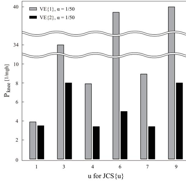
**Figure 4:** Stability region of the knee gain  $P$  for six JCS pairs. Each  $JCS\{u\}$  corresponds to the ones shown in Table 2. Gray and black bars represent two different viscoelasticity parameters shown in the top-left corner. The minimum  $P$  value was 0.1 for all conditions.
