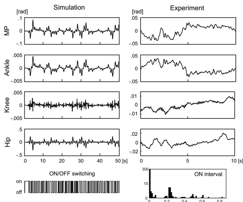
**Figure 6:** Joint angular displacements for simulation and experimental data. Left: time series for 50 seconds of the four joints' angular displacements obtained by simulation with Gaussian white noise. Intermittent switching of the active torque (on/off) is shown in the bottom. Right: experimentally observed four joints angular displacements during tiptoe standing for 10 seconds.
