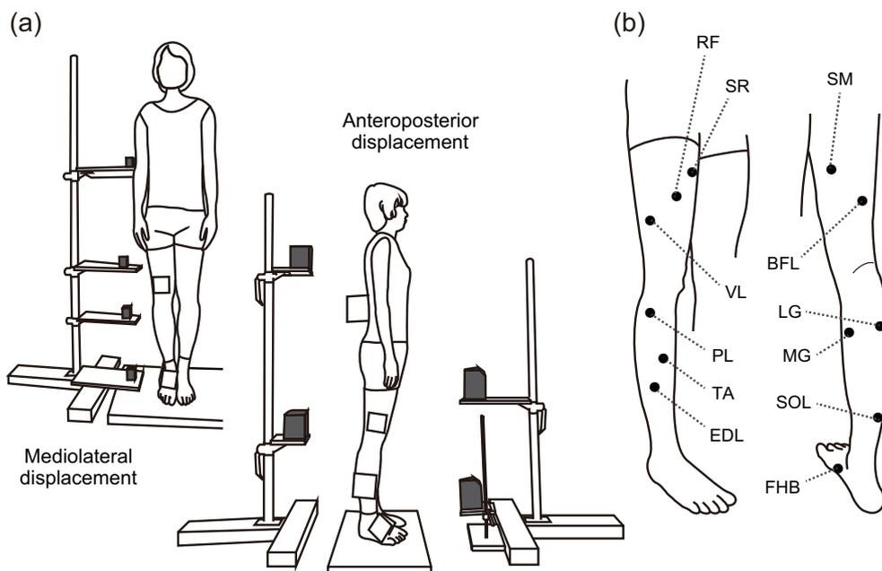
**Figure 2:** Experimental set-up and EMG location. (a) The displacements of the ankle, knee, hip, and ASIS were measured by eight laser sensors (small black equipment in front/side of participants). Laser lights were reflected at
