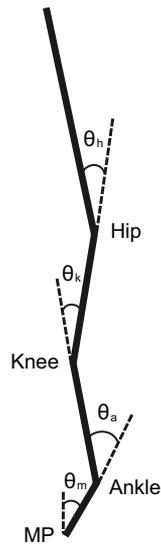
**Figure 1:** A quadruple inverted pendulum model. A model for a human standing tiptoe in the sagittal plane. Each of four links represent foot (MPankle), shank (ankleknee), thigh (kneehip), and HAT segments, from the bottom. Joint angles were defined as relative angles between adjacent joints except for joint angle of the MP being relative to the vertical line.
