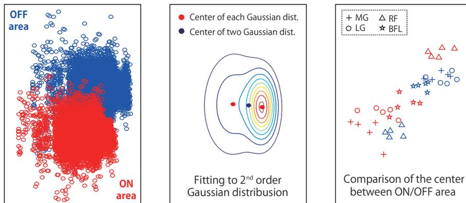
**Figure 2:** Mixed Gaussian distribution fitting of on/off area. Left: sample distribution of on/off area during a 120-sec trial. Middle: Example of a mixed (2nd order) Gaussian distribution. Two red points and one blue point represent each center of two Gaussian distributions and their center, respectively. Right: examples of the distribution of on/off centers in the knee torque plane for five
