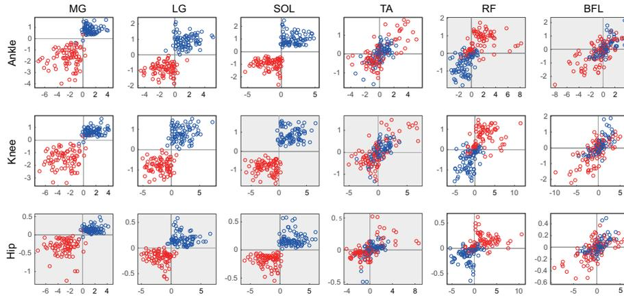
**Figure 4:** Centers of on/off area in the torque planes. Red and blue plots represent on and off area centers, respectively, of five trials from eight participants' both legs (80 samples in total for each figure). Top, middle, and bottom figures show distribution in the torque planes of the ankle, knee, and hip, respectively.
