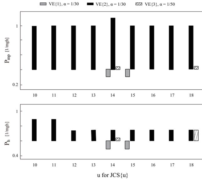
**Figure 5:** Stability region of the MP and hip gain  $P$  for nine JCS pairs. Top and bottom figures represent  $P$  regions for the MP and hip, respectively. Each  $JCS\{u\}$  corresponds to the ones shown in Table 2. Gray, black, and brace bars represent three different pairs of viscoelasticity and alpha shown on the top.
