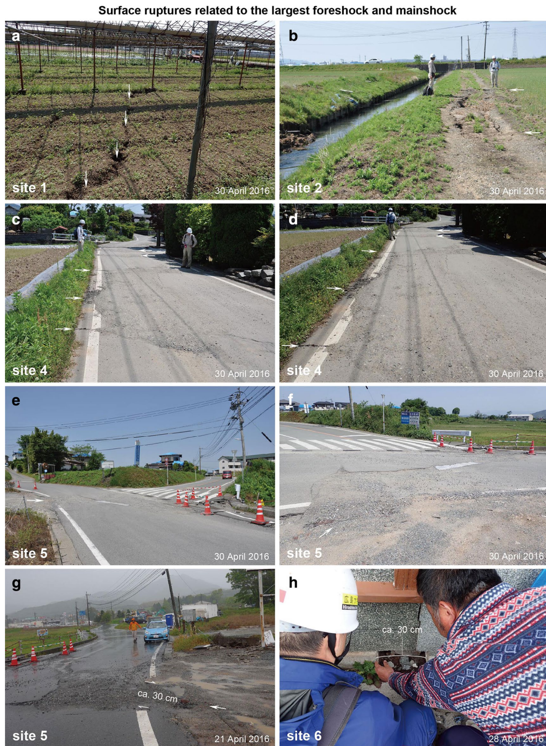
Fig. 4 Snapshots of surface ruptures related to the largest foreshock and mainshock at each site shown in Fig. 1c and/or Fig. 2. a Mole-track structures and open cracks, which first appeared associated with the largest foreshock and later enlarged due to the mainshock. b Two fault traces on an unpaved road, indicated by white arrows , between which a small depression appeared. Vertical offset of ca. 10 cm up on the north was identified across the two fault traces. c, d Five rupture traces with right-lateral offset of a paved road. Total amount of offset was 13–14 cm. e–g A fault trace on a paved road with right-lateral offset of ca. 30 cm. h An open crack of a concrete block, whose width was ca. 5 cm after the largest foreshock and ca. 30 cm after the mainshock
