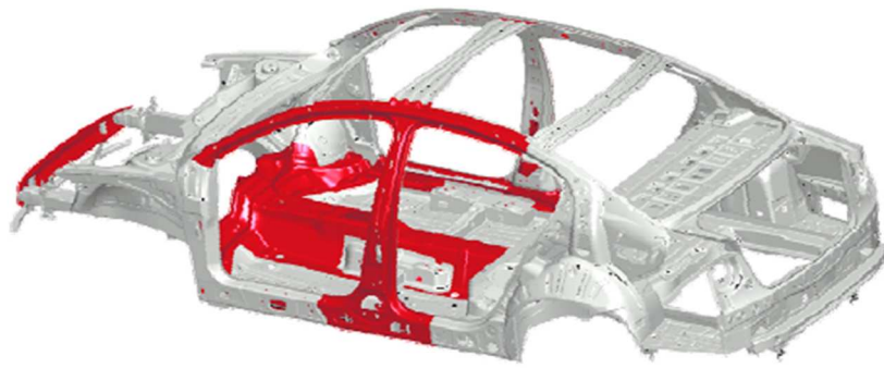
Fig. 1-10. 6 th Volkswagen Passa; integral ultra-high steel (UHSS) design of the passenger compartment (source: Volkswagen AG) 34 .
