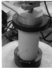
Figure 2. Samples failure plane of UCS test
