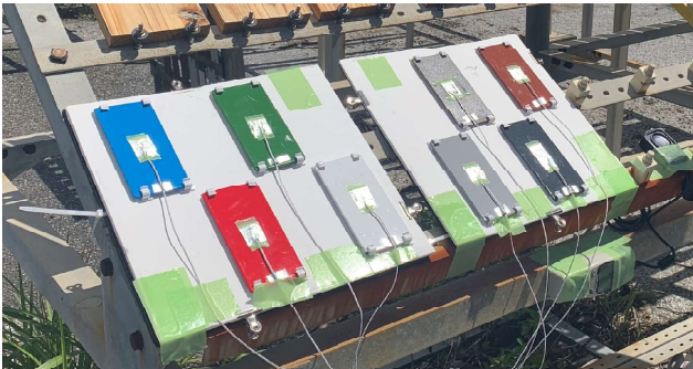
Fig.3 Steel specimens painted with different colors in Nago, Okinawa
