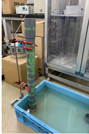
Figure 5.3: Schematic setup of the soil column method.
