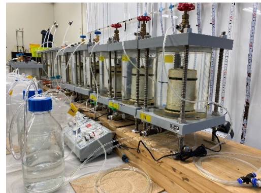
Figure 4.1: Column test in a) schematic details of the flexible wall permeameter and b) appearance of the test setup.
