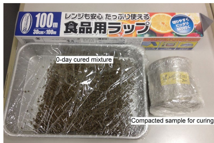
Figure 3.3: Photo of a compacted soil sample prepared for the curing step.
