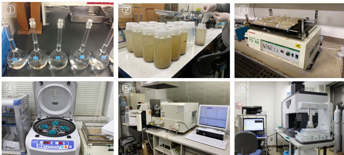
Figure 3.4: Pictorial representation of typical steps for batch-type test showing 1) preparation of arsenic solutions, 2) adding soil samples to solution, 3) shaking step, 4) centrifugation step, 5) analysis of arsenic amounts using atomic absorption spectrophotometer and 6) analysis of water-soluble ion amounts using inductively coupled spectrophotometer.
