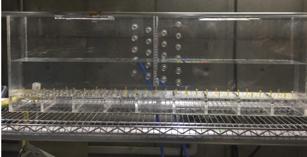
Figure 3 - 13 Arrangement of needle system for the rainfall application
