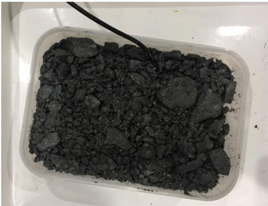
Prepared the specimen with sensor (Saturation = 55%)
