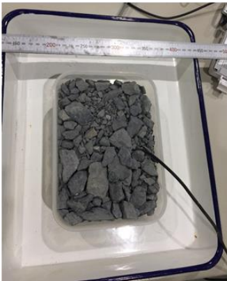
Prepared the specimen with sensor (Saturation = 0%)
