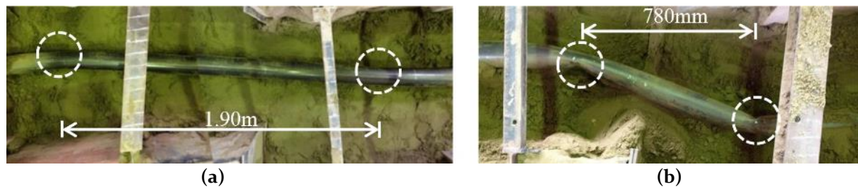
Fig. 3.6. Experimental results of pipeline crossing strike-slip fault with angle of 90°: (a) buried in soft soil, (b) buried in hard soil [21].
