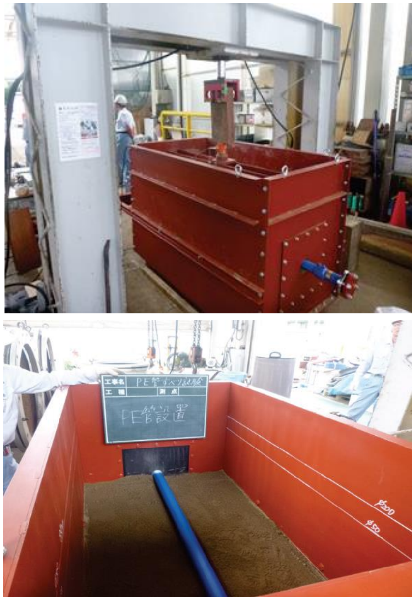
Fig. 7.23. Push-in experiment for 63 mm HDPE pipeline buried in dense sand (95% compacted sand) by Nishikawa 2017 [42].
