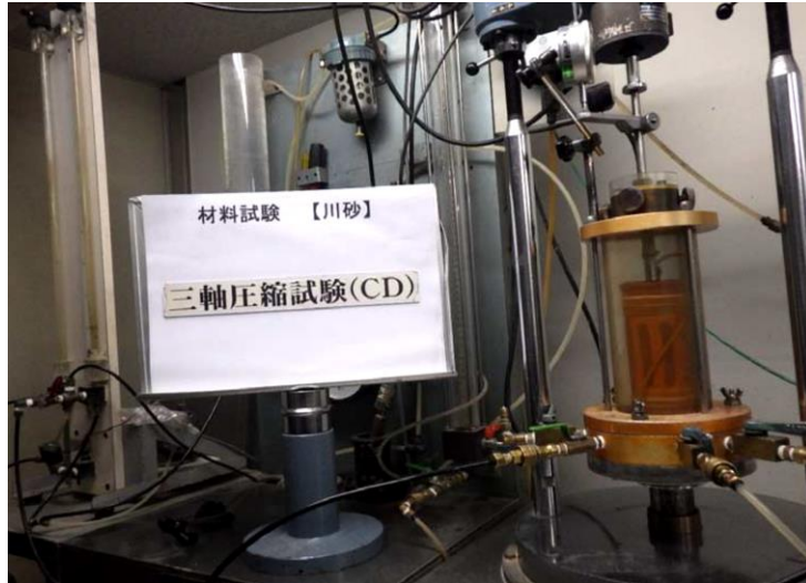
Fig. 7.7. Triaxial shear test (CD) photograph.
