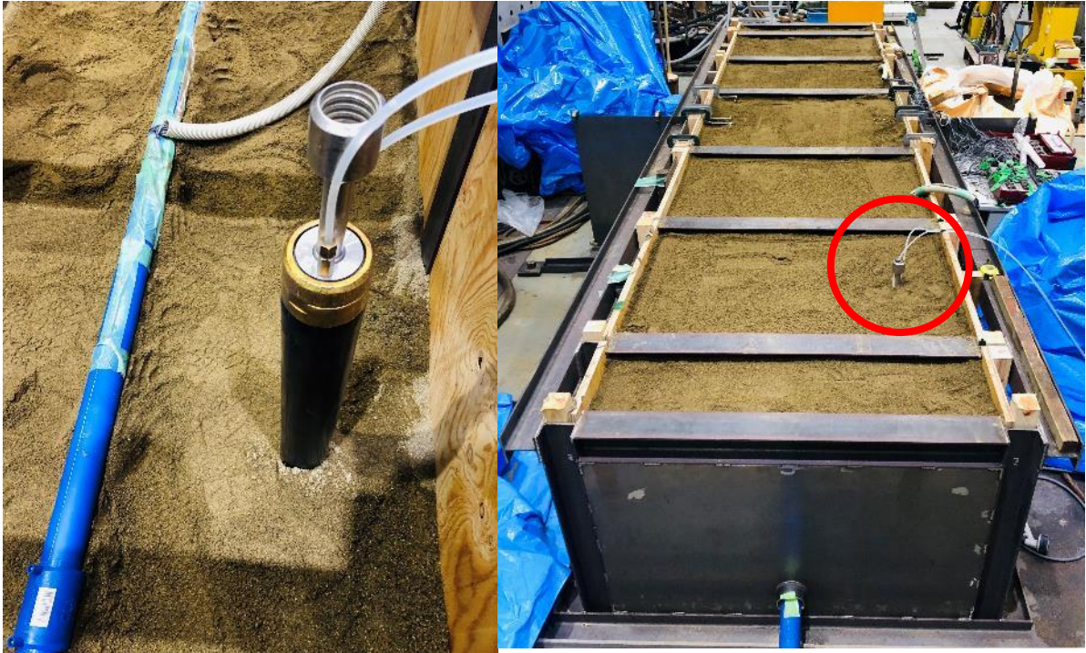
Fig. 7.9. Lateral load test (LLT) inside the split-box, before faulting.
