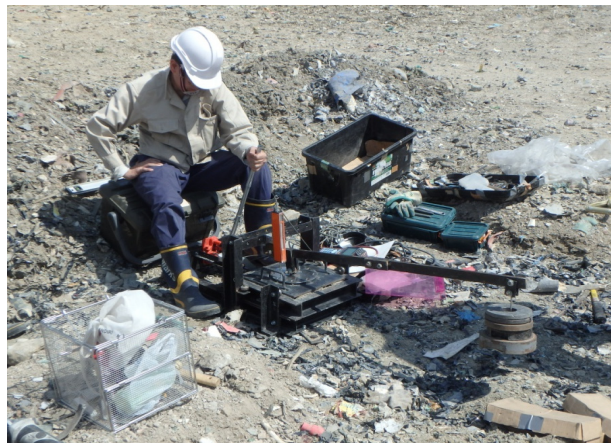
Figure 5.3 In-situ direct shear test
