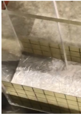
Figure 5.12 Installing fiber-sand mix layer for centrifuge model
