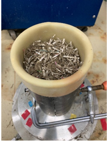
Figure 3.25 Specimen for triaxial test
