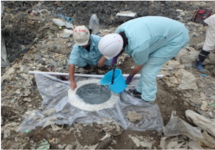
Figure 3.3 In situ wet density test
