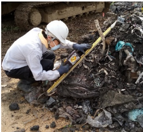
Figure 5.2 In-situ repose angle test
