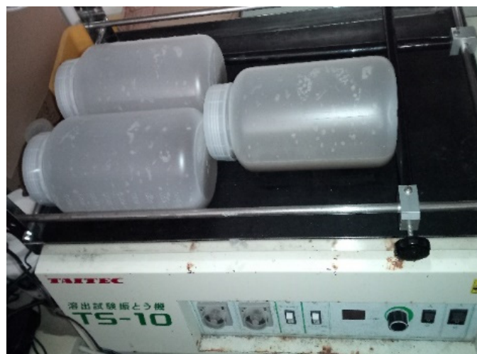
Figure 4.17 Laboratory batch leaching test
