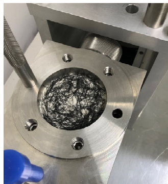
Figure 5.9 Preparation of specimen for direct shear test
