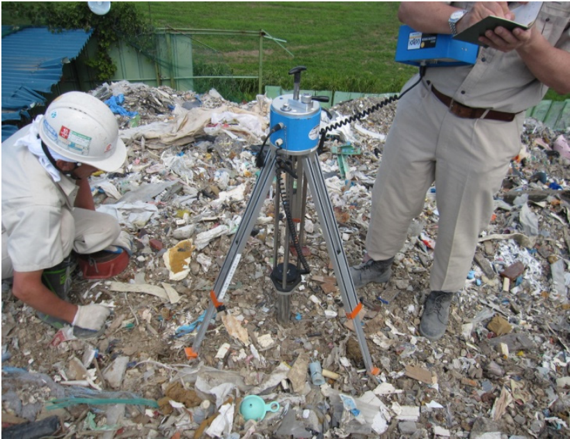
Figure 3.5 CASPOL impact value test
