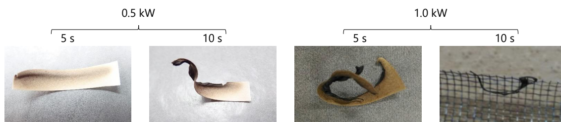
Figure 6-8. Photographic images of cellulose chars obtained under various fast pyrolysis conditions.
