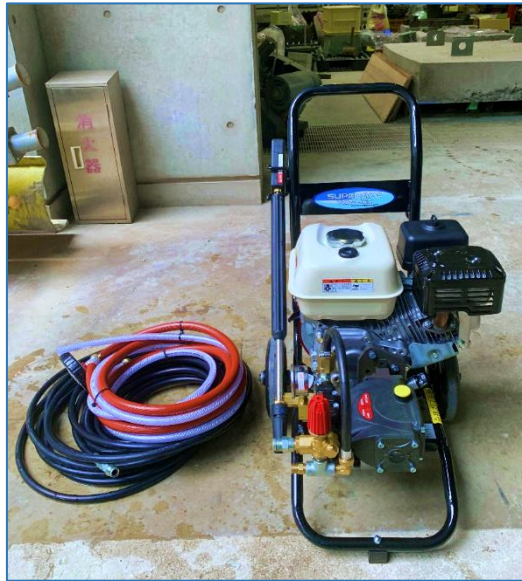
Figure 3.10 Power washer equipment
