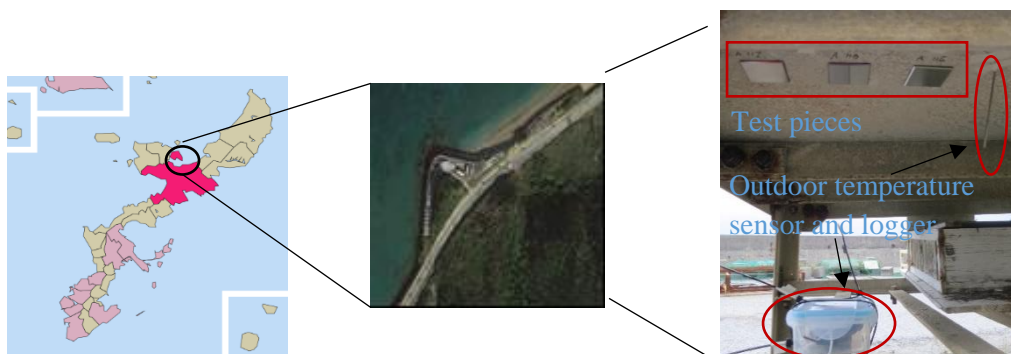
Figure 2.13 Specimen installations in Nago City, Okinawa, Japan
