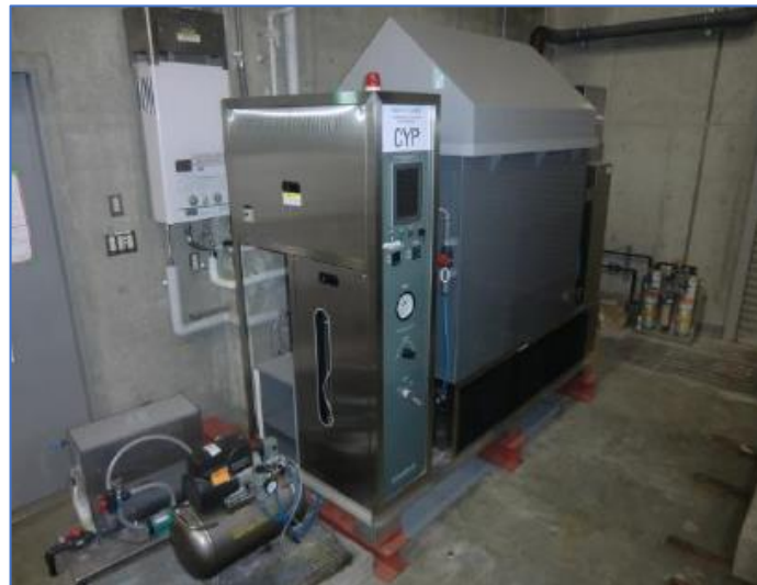
Figure 3.1 Combined cycle corrosion test instrument
