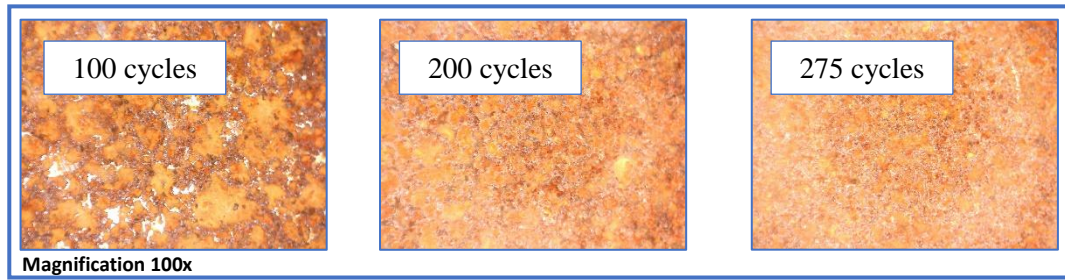
Figure 3.14 Rust color changes of SMAW steel in 0.05% salt solution test
