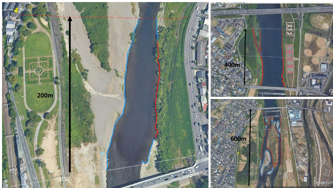
Fig. 4-5 Shoreline length of three different reaches, left one is the downstream of No.5 weir, top right is the upstream of No.1 weir, and the last one is the downstream of No.1 weir.
