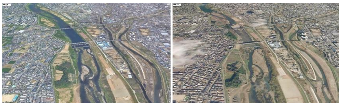
Fig. 5-1 Satellite images of before(2019) and after No.1 weir removal (2021), note that the upstream gravel bar exposed after removal.
