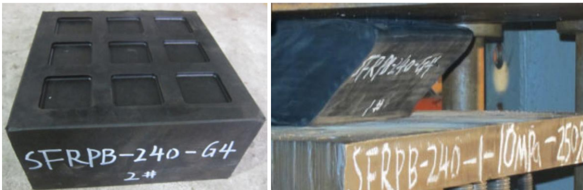
Figure 2.4 PFRI isolator made and tested by Tan et al. (2014)
