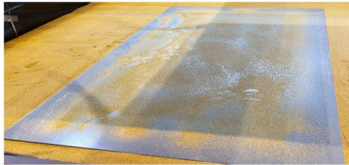
(b) Deposition of sandwiched sand and (c) bottom PVC surface after sand deposition
