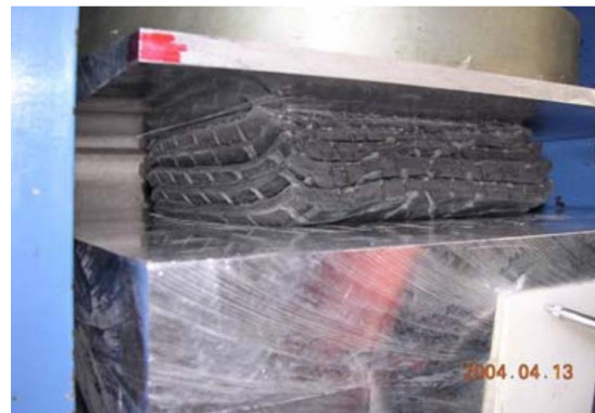
(b) Inclined compression test setup
