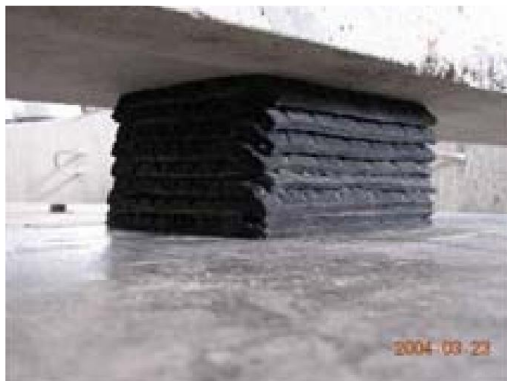
(a) Stacked STP specimen
