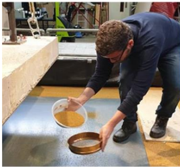
(b) Deposition of sandwiched sand and (c) bottom PVC surface after sand deposition
