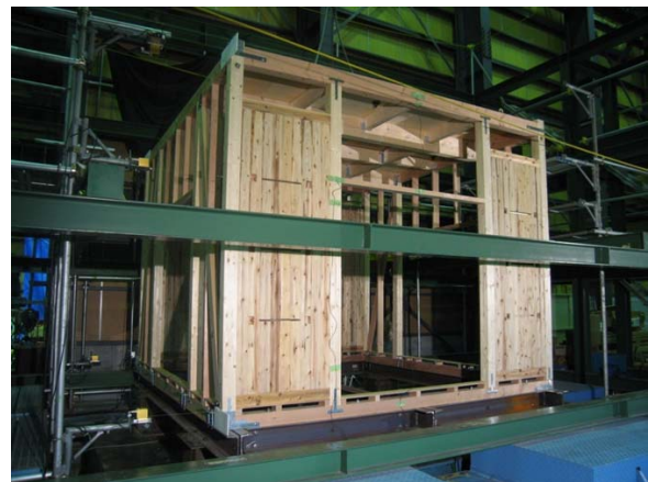
Photo 3 A specimen for a shaking table test of a one-room wooden house model with “Wall-of-Columns” reinforcements.
