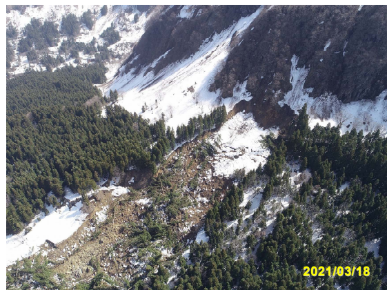
Fig. 9 A landslide that traveled a long distance in the early stage of snowmelt period during strong winds.
